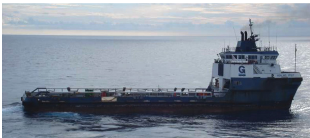
The ship is a Platform Supply Vessel built in 1999 with two Caterpillar 3606 main engines (4640BHP; LOA 66m; DWT 2800mt). The vessel is classified by ABS.
