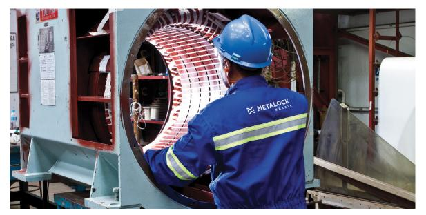
The generator was tested at nominal rpm, at no-load, short circuit and 233.8 KVA inductive load, also the output voltage has been checked with the generator self-excited. After the workshop test the generator has been returned to METALOCK for dismantling and preparation, to be transported to the vessel. The Stator and the Rotor were separated and packed in two wooden boxes.
